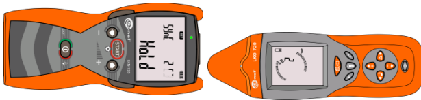
Fig. 5 Positioning the transmitter and receiver during synchronization
